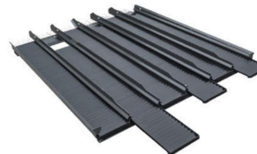
In very damp harvesting conditions, a clean preparation floor always ensures high throughput rate and optimal threshing quality. That's why the preparation floor of the Fendt L-Series is easy and convenient to remove.
