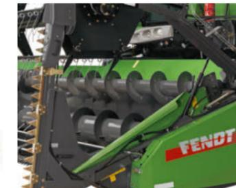
The optional rapeseed auger increases the crop flow to the crop elevator in high crops and enables an increased throughput rate.
