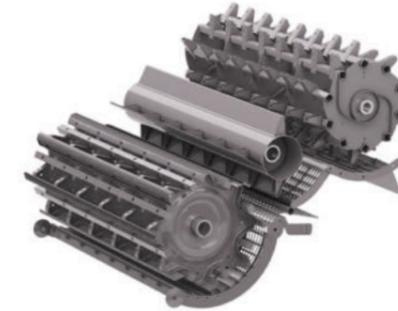
The separator concave is completely above the Multi Crop Separator. This setting is recommended primarily for crops that only require light threshing and in dry conditions.
