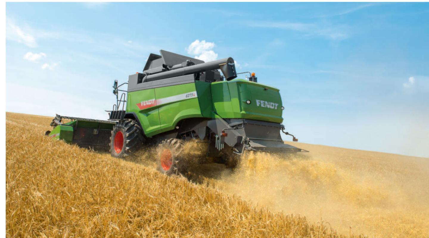
Operators can switch quickly and easily between swathing and chopping modes, simply by moving a lever.
