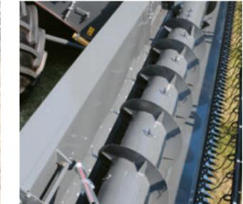
The Power Feed Roller guides the crop very uniformly from the table into the crop elevator.
