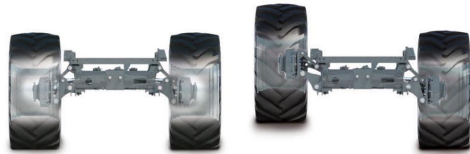
Easy switching between work and transport mode using the ParaLevel system, which compensates for slopes up to 20%.
