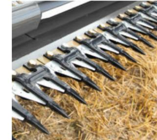
The FreeFlow table has feed fingers over the entire width, which increase the throughput of the intake auger and guarantee active, fast feed into the crop elevator.
