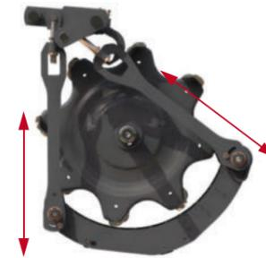
The separator concave is rotated under the Multi-Crop Separator (MCS). This setting improves the separation performance in long straw and wet conditions, enabling high output, even under difficult conditions.
