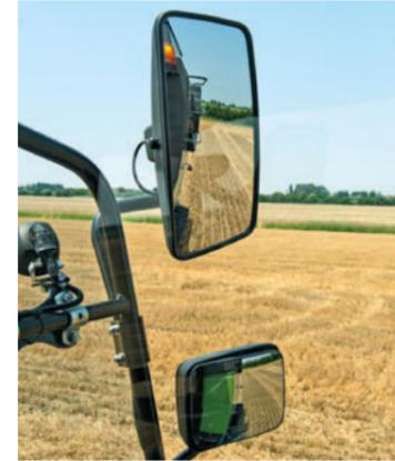
A clear view to the table and stubble, and to the spreading pattern of the straw chopper with the camera, enables the best performance in the field.
